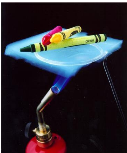
Figure 1: Crayons supported on an aerogel over a flame
